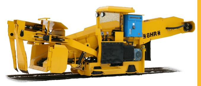
The railborne Gialoader are electro-hydraulic driven loaders with a unique dual digging arm system designed to operate efficiently in narrow or limited work areas.
