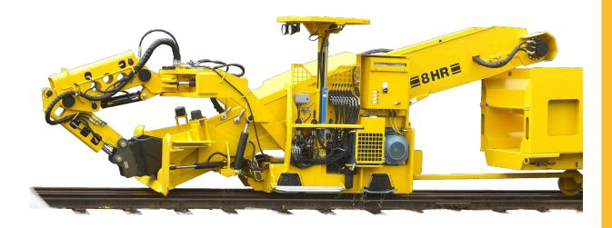
The railborne Gialoaders are electro-hydraulic driven loaders with a back-hoe digging arm system designed to operate efficiently in narrow or limited work areas.
